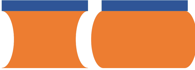
Figure 4.2: Examples of over (a) and under (b) etching errors from a side-on perspective. In both cases the sample has been left in the etchant for an improper amount of time, leaving behind too much or too little copper. Whilst generally small, some designs with low ratios of copper to empty space can fail completely as sections near the edge of the design begin to over-etch and sections near the middle remain under etched.
