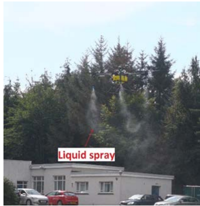
Figure 1: Crop spray drone hovering. The liquid spray is seen below the drone.
