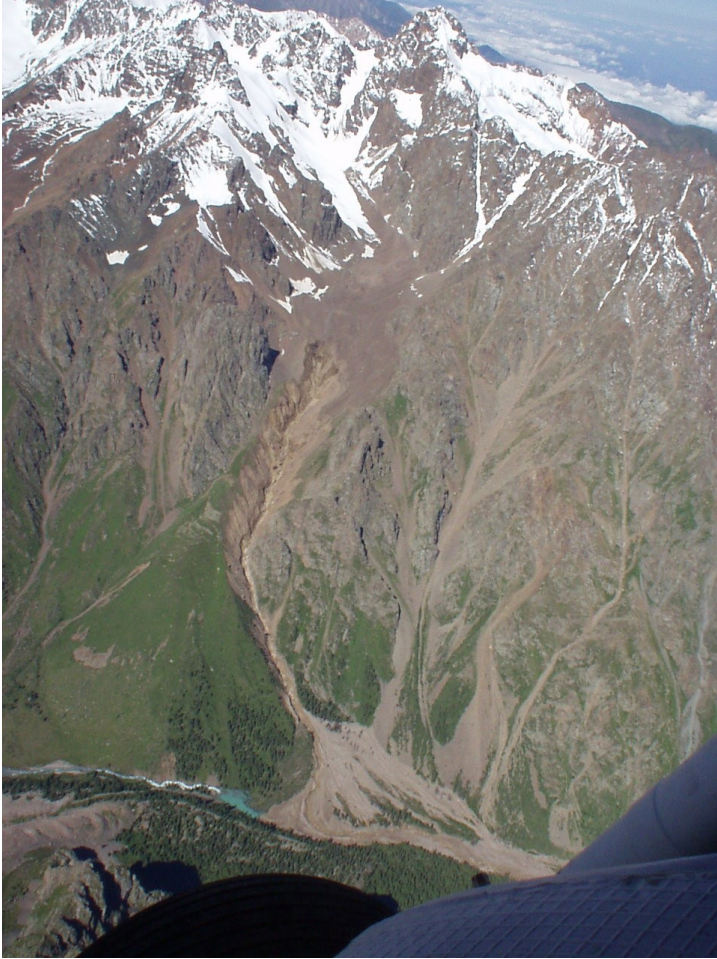
Figure 34 The 2003 debris flow in Left Talgar Valley (Ile Alatau, Tien Shan, Kazakhstan) originated from a degrading rock glacier front. Photo: Institute of Geography, Almaty.
