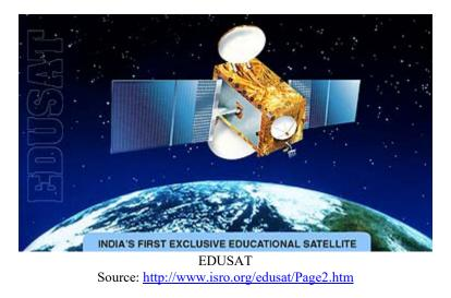
The satellite has multiple regional beams covering different parts of India - five Ku-band transponders with spot beams covering northern, north-eastern, eastern, southern and western regions of the country, a Ku-band transponder with its footprint covering the Indian mainland region and six C-band transponders with their footprints covering the entire country.
