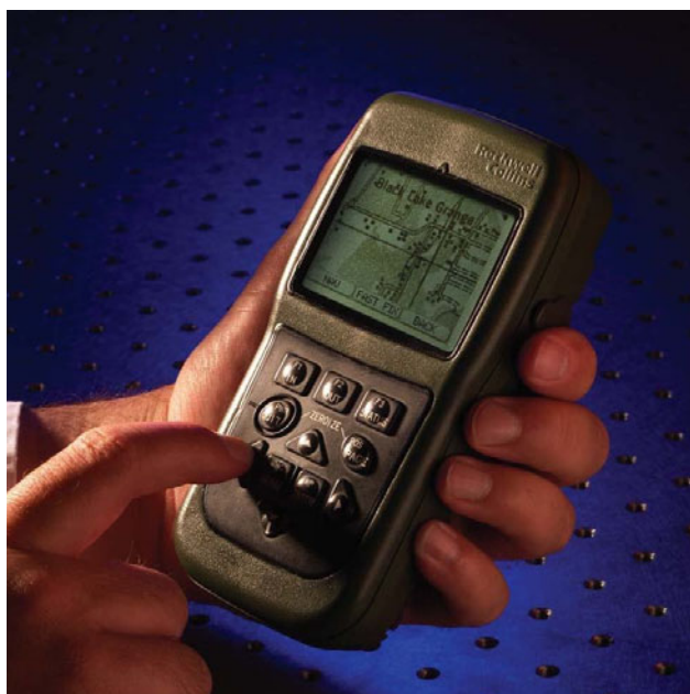
Figure 1. Users can view raster maps and vector maps on DAGR's situational awareness and moving map display.
