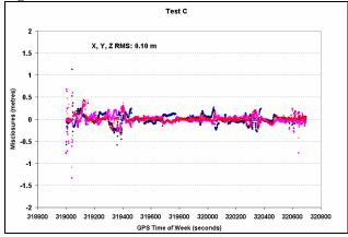
When the post update corrections are applied, the relative position errors for tests A, B and C are 0.05m, 0.07m and 0.10m respectively. The RMS of all the tests with the post update correction is 0.075m, which compares favorably to
