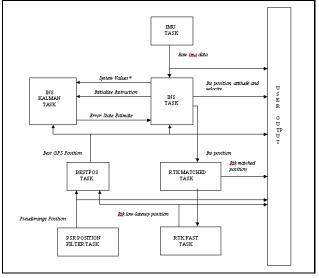
The Kalman filter has 15 basic states including nine for position, velocity, and attitude and six to model gyro and accelerometer biases. This is described in [2]. An additional six states are included to model GPS antenna offset errors and the previous position error vector [3].
