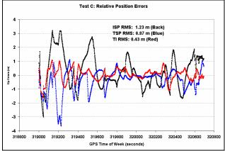
The previous figures 8, 9 and 10 show north, east and up component position errors for tests A, B and C respectively. Each has three sets of points, black being the ISP systems, blue showing the TSP systems and red depicting the TI systems. The transferred inertial (TI) method shows the best results of the three. A summary of the RMS values of all the position components for all the methods is shown in the following table 3.
