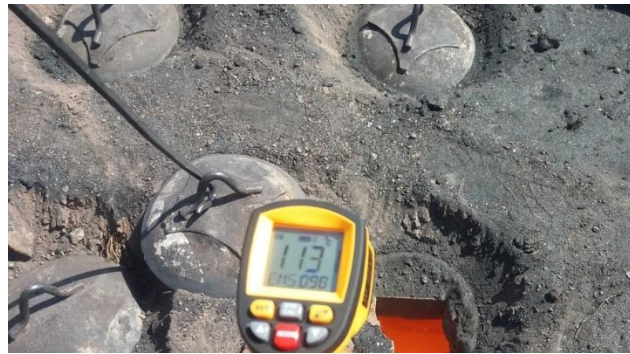
Figure 9. measuring the temperature of the brick Kiln by infrared thermometer
