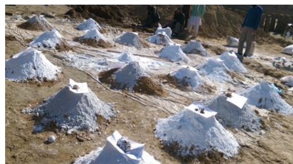
Figure 7. Marble dust and clay in the mixed form set for making bricks
