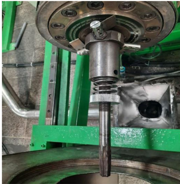
Gambar 1. As Cutting Terpasang di Mesin Extruder
