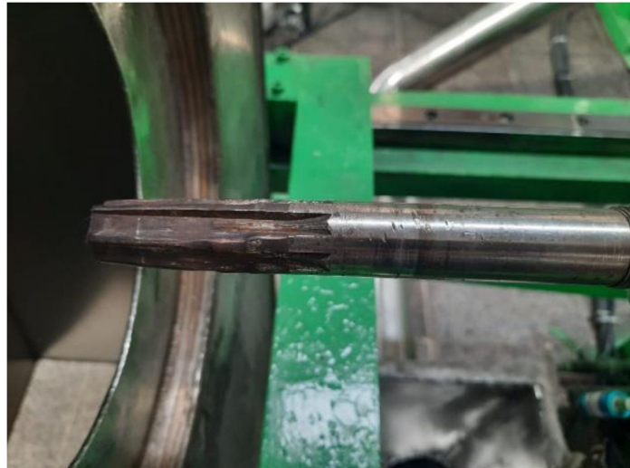
Gambar 2. As Cutting Pada Mesin Extruder Twin Screw
