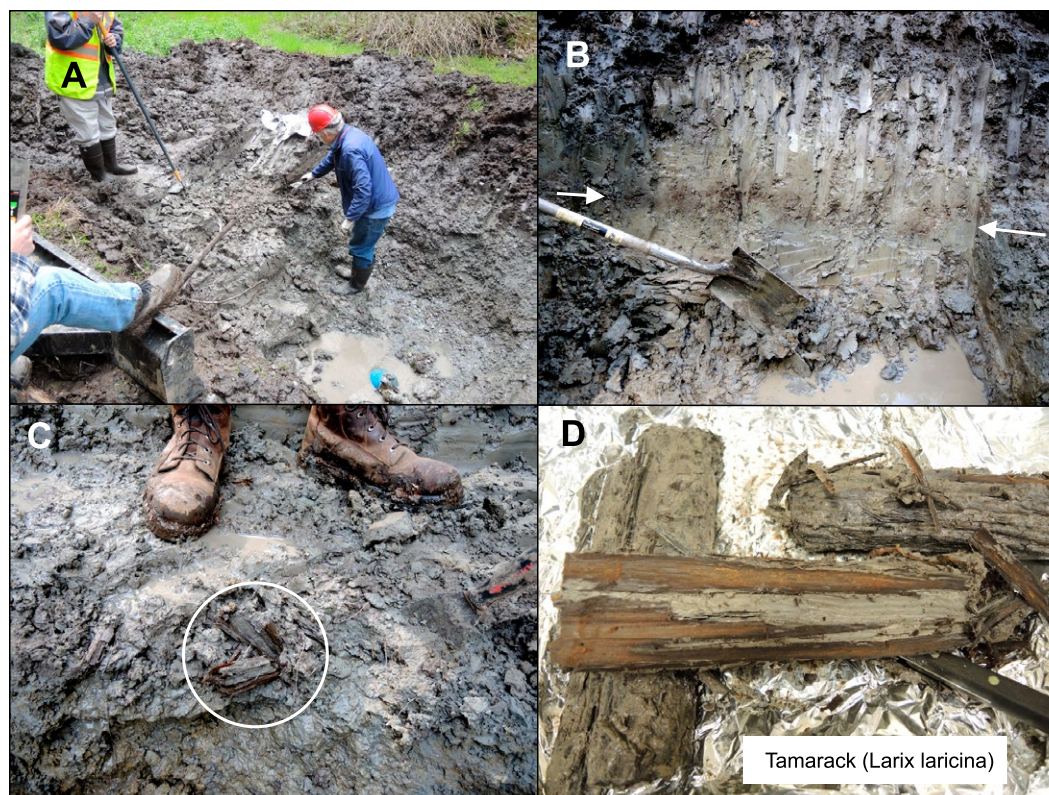
Figure 17. Kettle excavations at Pit 2 as located by number on Figure 16. (A) Removal of Tamarack wood samples onto aluminum foil. (B) Dark organic and wood layer in shallow clay-rich till zone between arrows. (C) Close-up of Tamarack wood fragments prior to removal from organic layer. (D) Compressed Tamarack wood specimens after splitting to show impregnation by clay extending through interior of samples due to inferred ice pressure. Knife handle is 1.5 cm wide.
