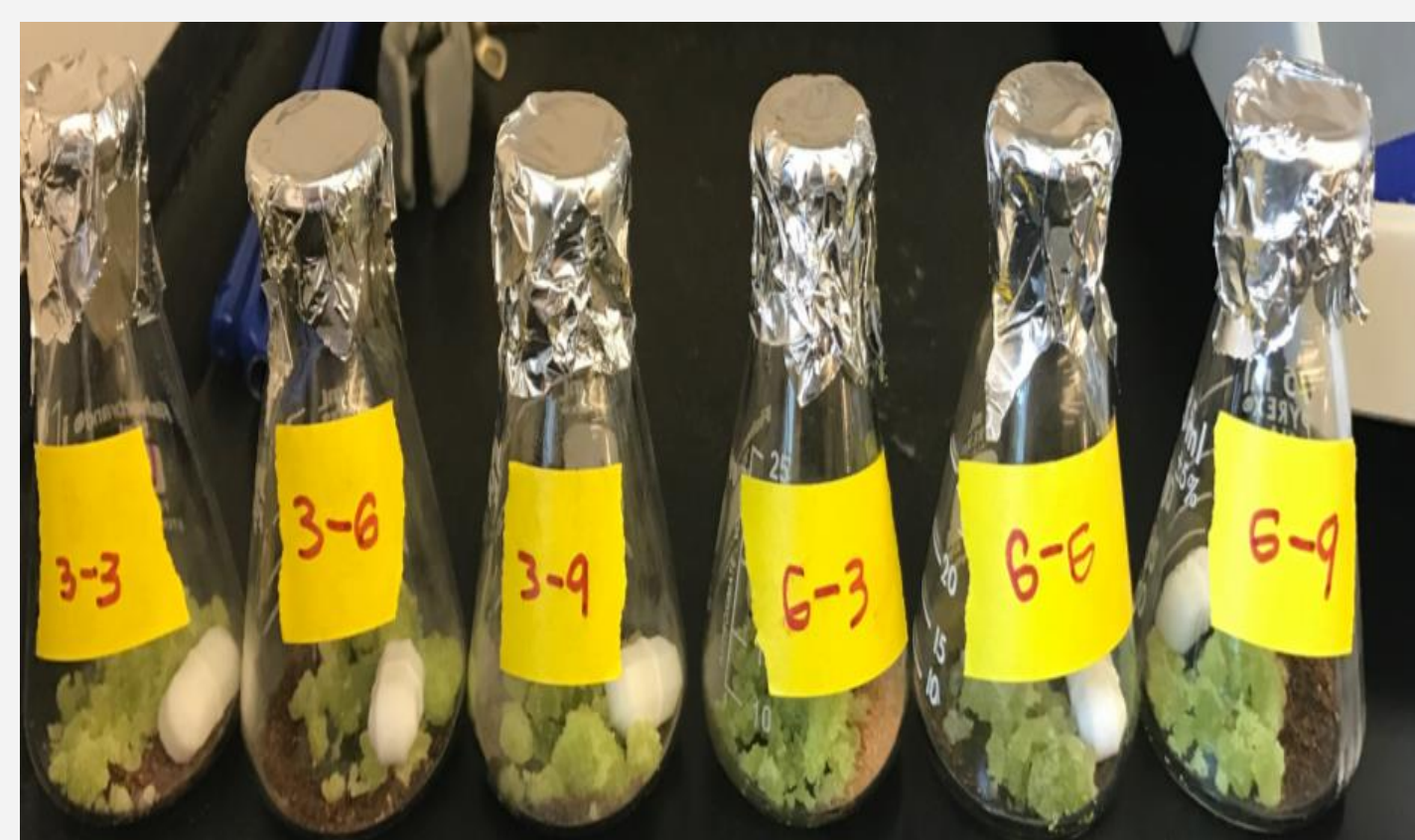
Figure 1. Samples labeling: the first being the amount of time that the sample spent after subjection to the ionic liquid and the second number indicates the time spent in the mineral oil bath after treatment with 0.5 M hydrochloric acid.
