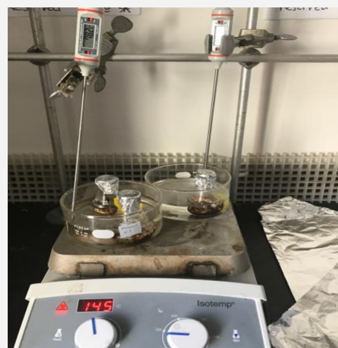
Figure 2. Samples are heated in a mineral oil bath for 3,6, or 9 hours at 80 degrees Celsius. A magnetic stirrer is added to completely mix the mixture
