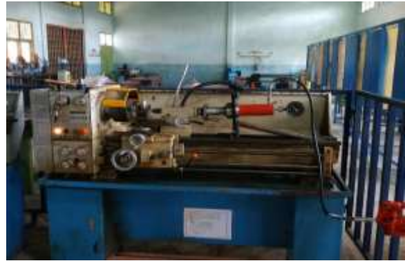
Figure 3. A turning machine was used for friction welding process
