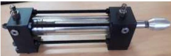
Gambar 12. *Double Acting Cylinder* transparan
