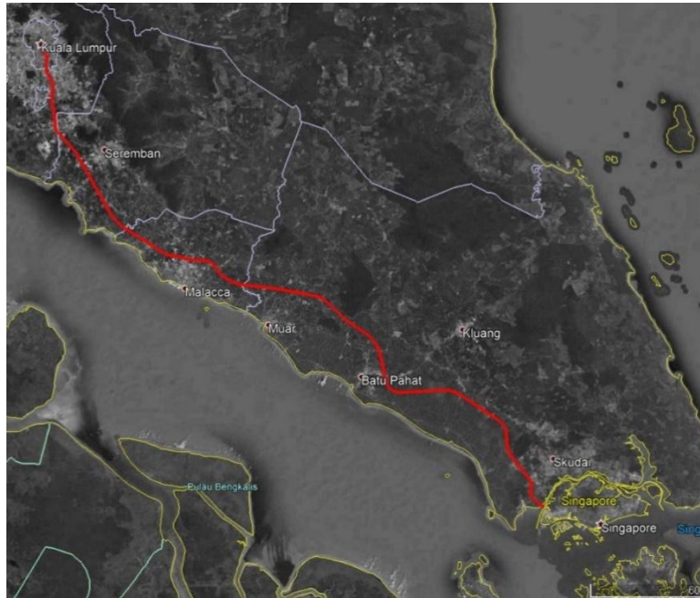
Fig.1: KL-SG HSR alignment (within Malaysian Peninsular only)
