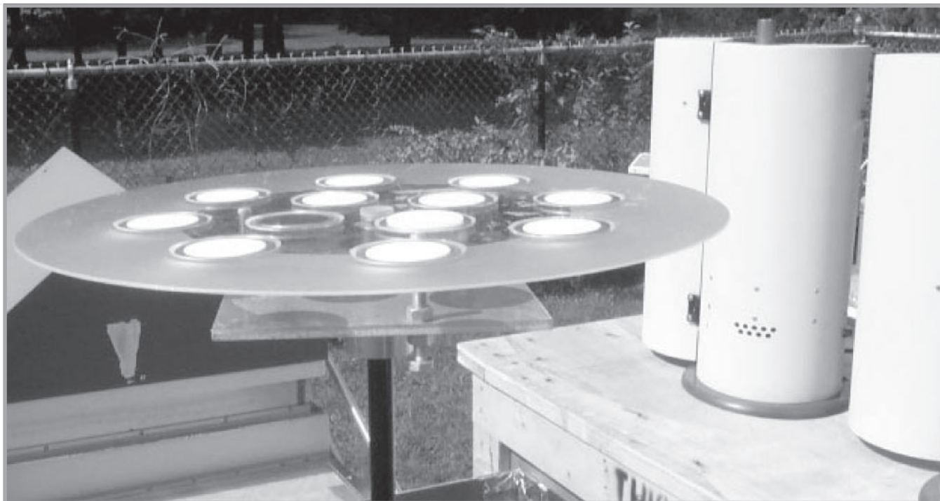
Figure 2. Knife-edge surrogate surface on top of the actuator. The white disks are the sampling media.
