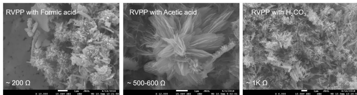
A.10: SEMs of RVPP-PEDOT synthesized from 1 M H 2 SO 4 rust via formic acid, acetic acid and carbonic acid.
