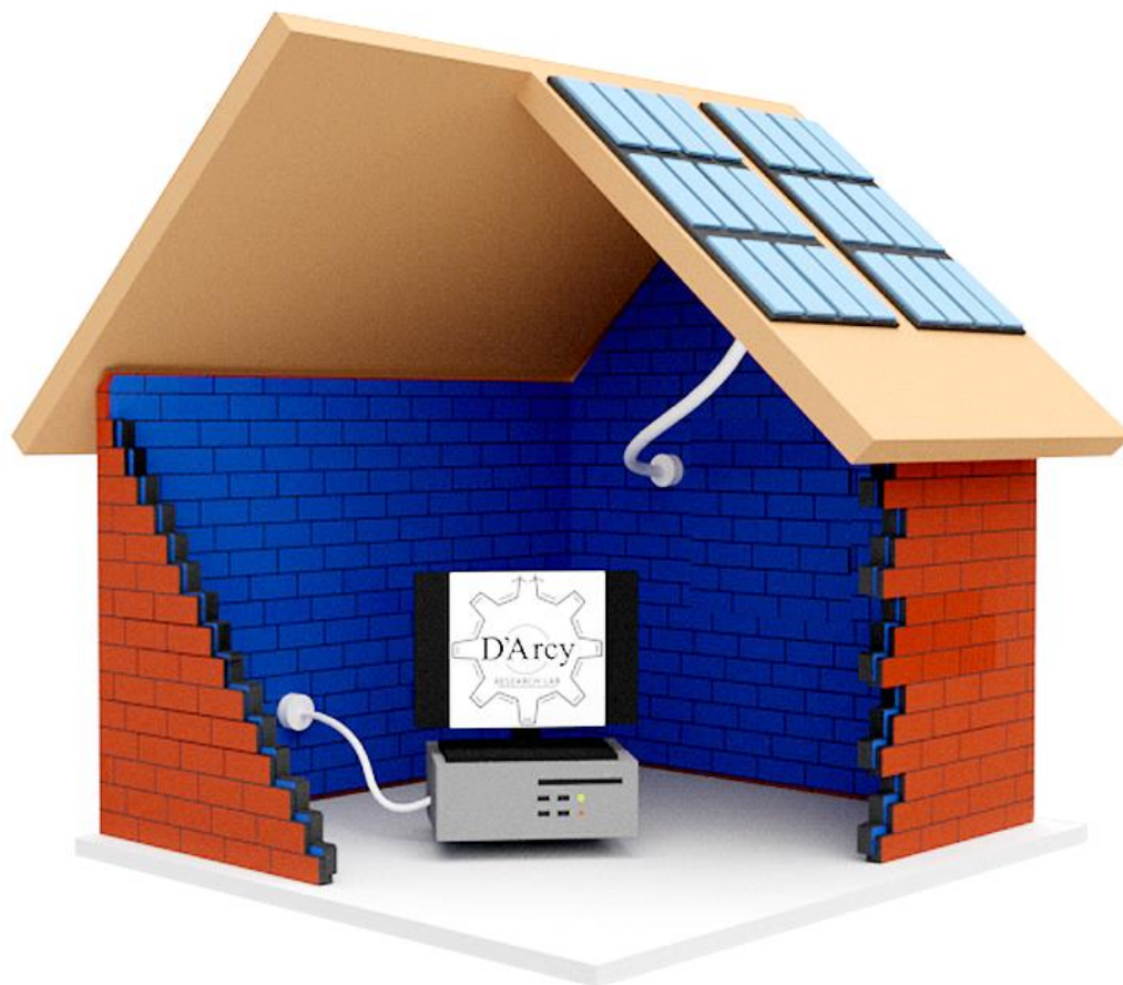
E.2: Schematic illustration of conductive brick for energy storage application
