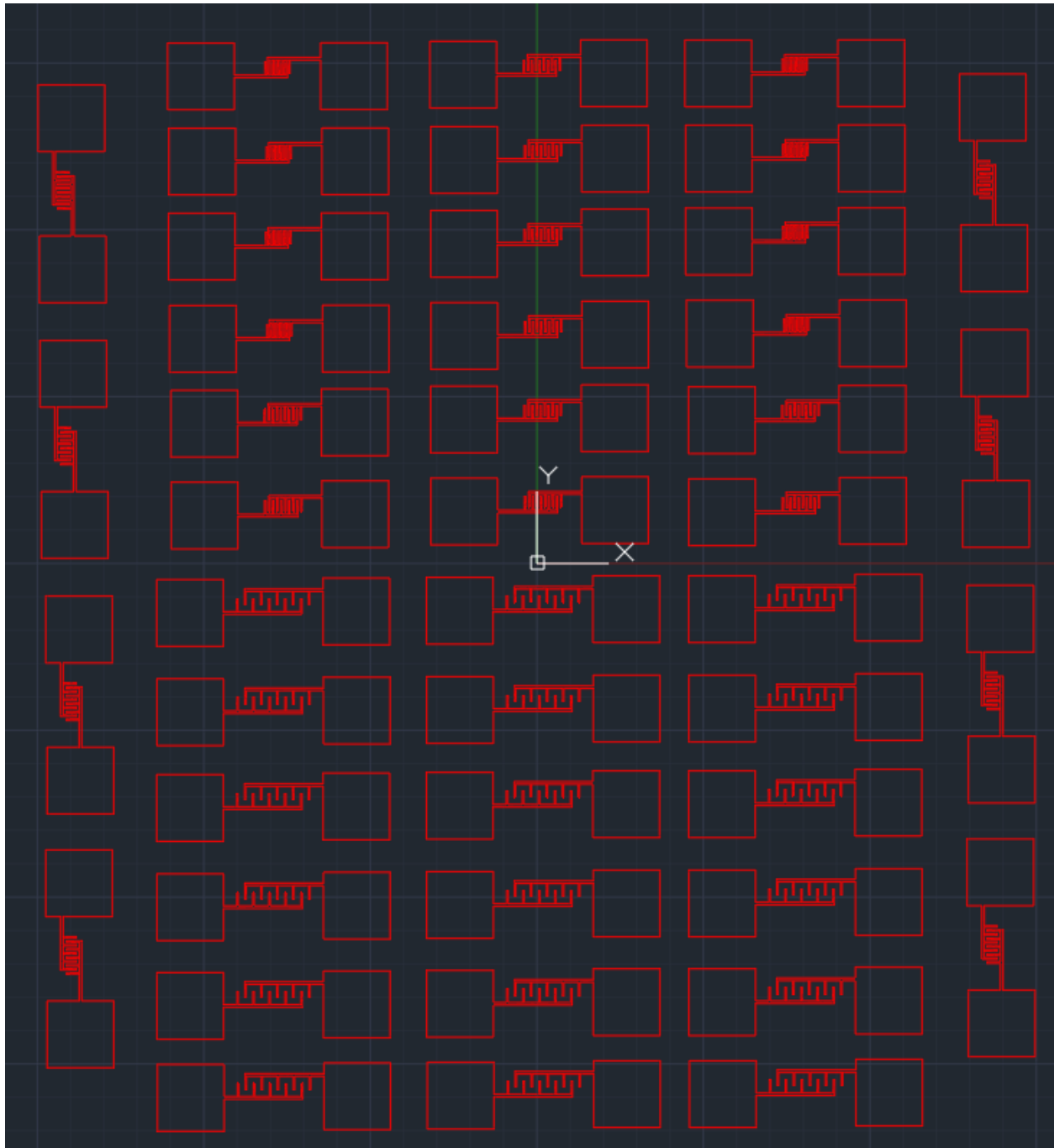
G.2: AutoCAD of small-interdigitated electrode microsupercapacitor.
