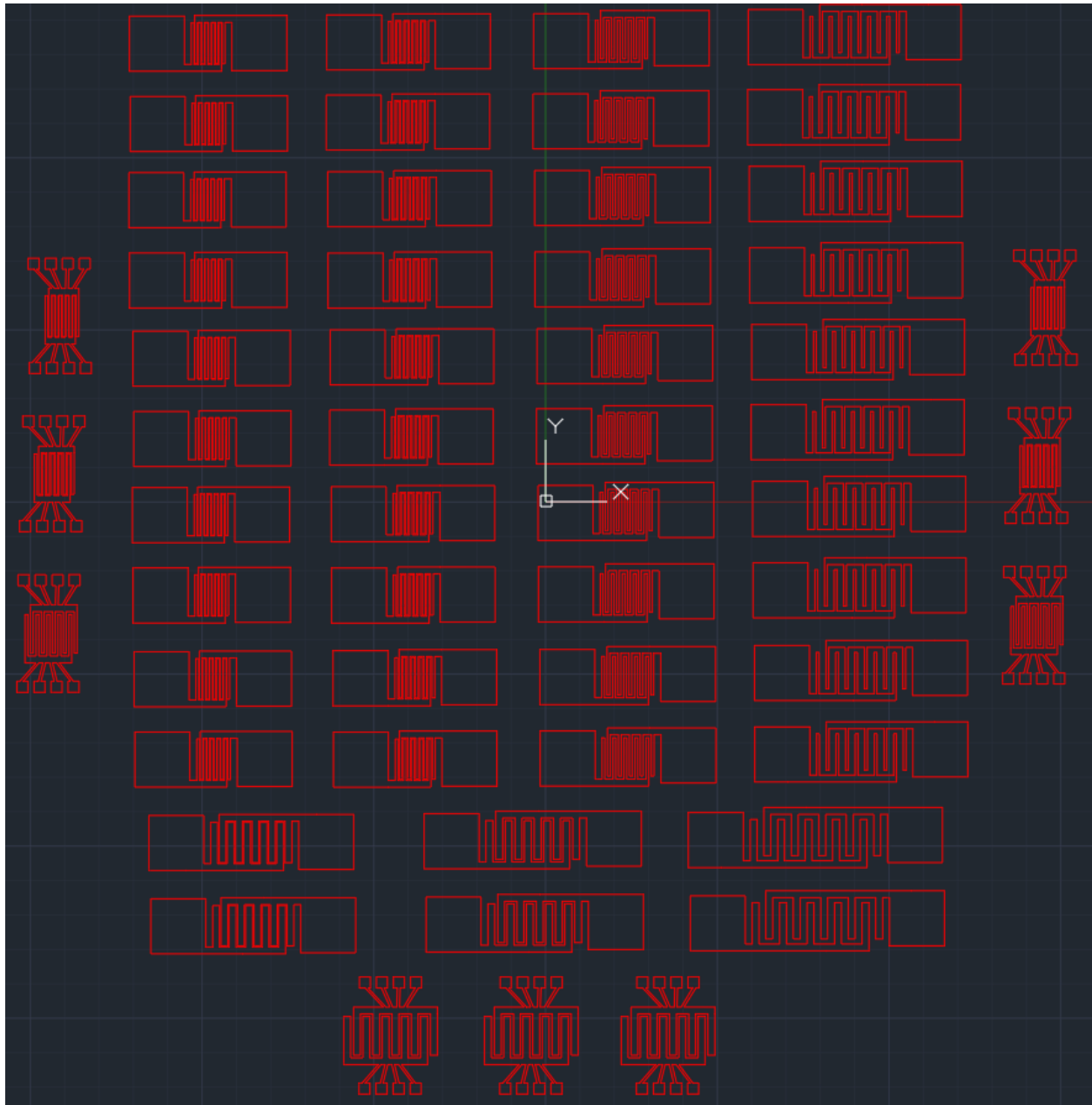
G.5: AutoCAD of large-interdigitated electrode microsupercapacitor and conductivity measurement pattern.
