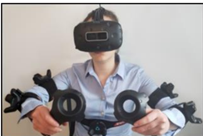
Figure 3.4. A subject donning the Vive trackers on the limbs (upper arm and forearm) and chest with Vive controllers in hand.
