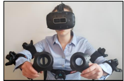
Figure 2.4. A subject donning the Vive trackers on the limbs (upper arm and forearm) and chest with Vive controllers in hand.
