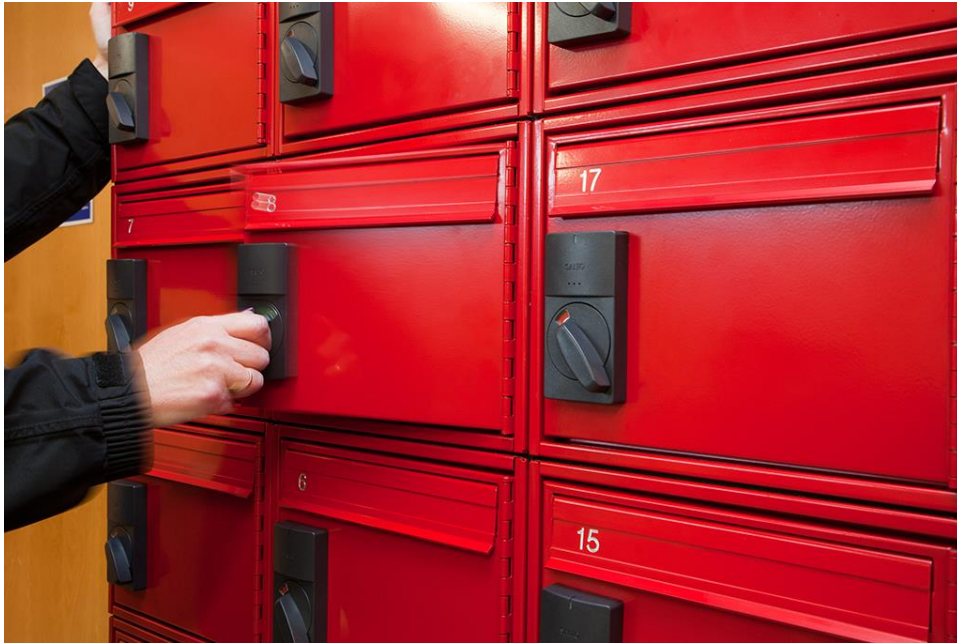
Figure 1: This system uses a PO box style setup with an RFID access card swiped to unlock the box. This would allow students to securely access their own homework in an electronically controlled box.
