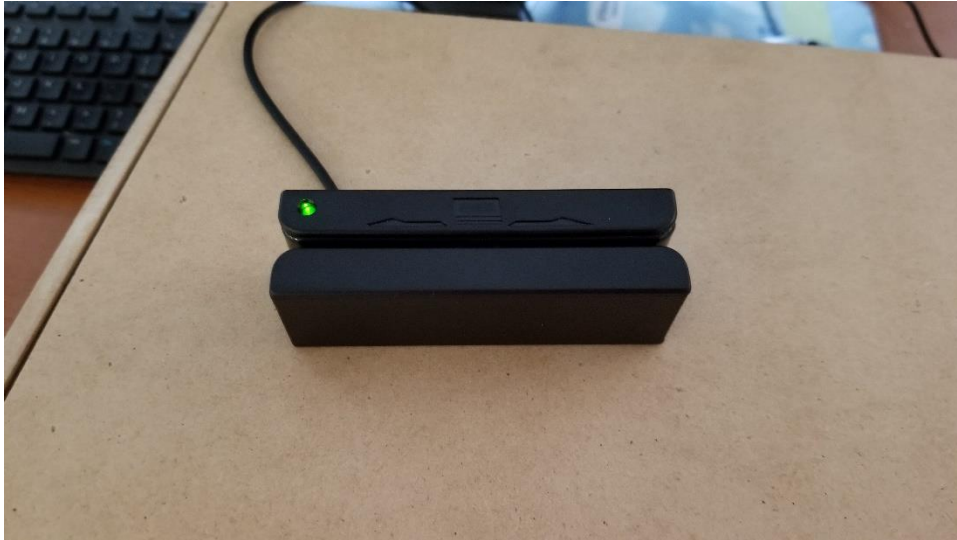
Figure 23: The card reader reads the student ID number off of the student ID
