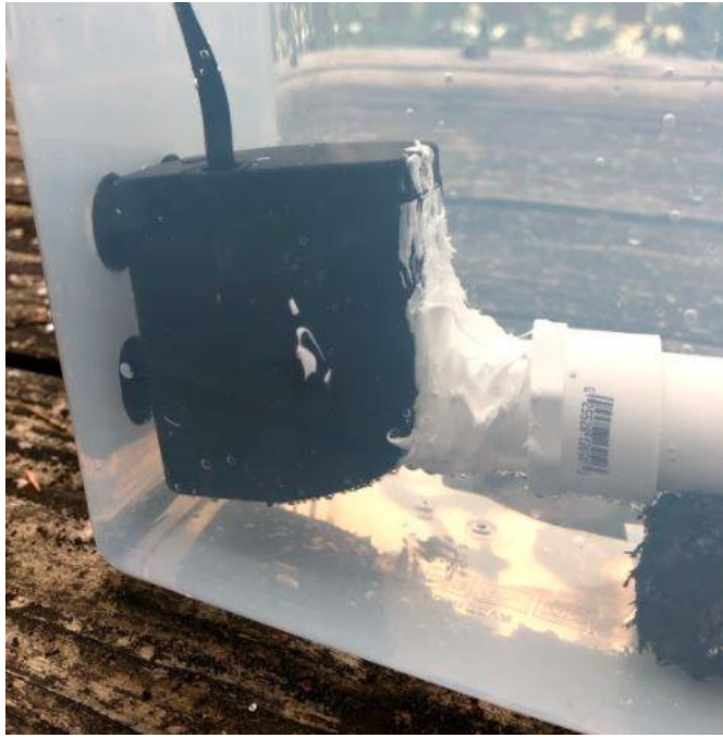
Figure 28- Submerged Pump in Lower Reservoir
