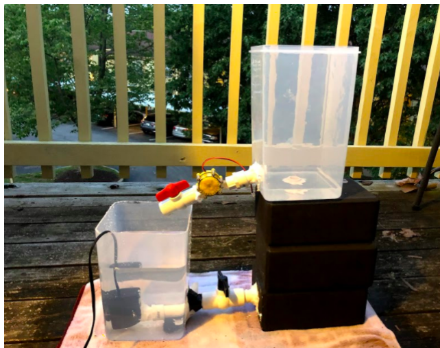
Figure 25- Image of entire pump hydropower storage prototype
