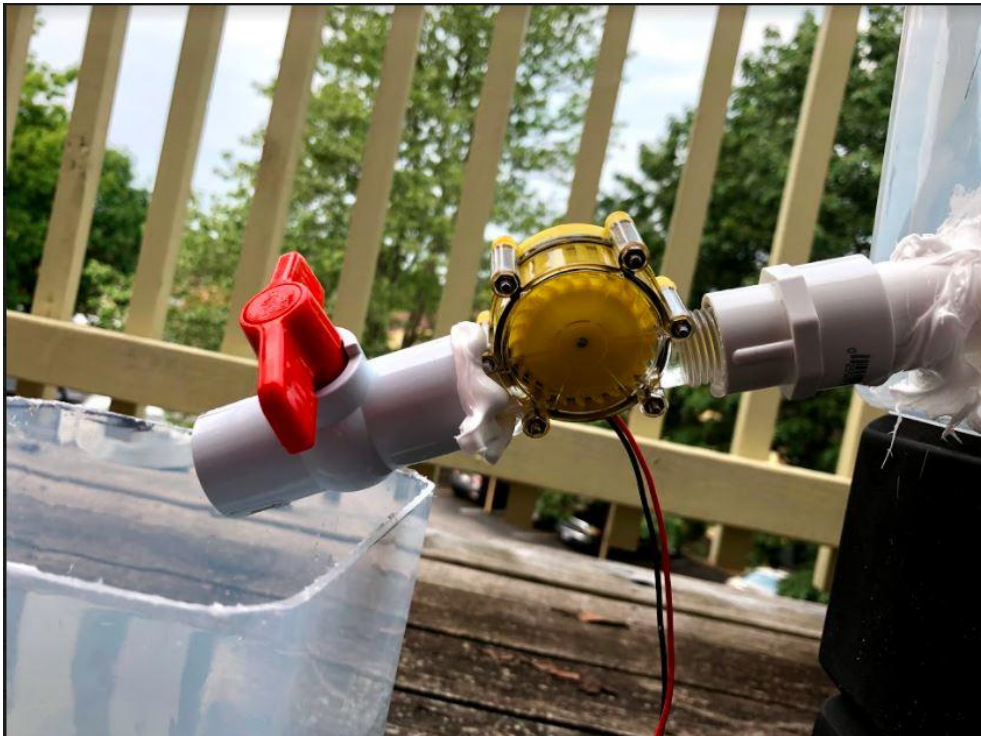
Figure 27- Turbine Generator and Valve
