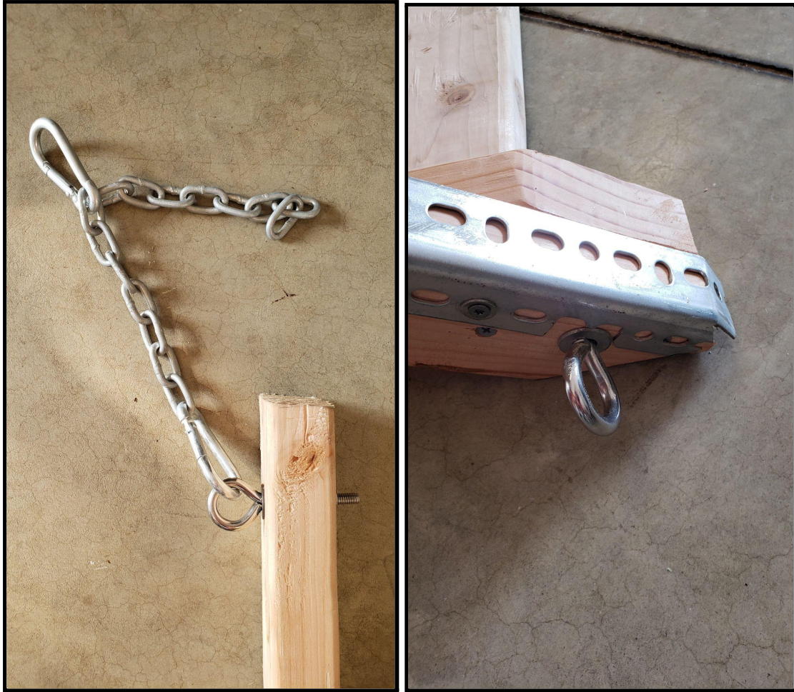
Figure 23: The eye bolts on the station and platform with the chain and spring locks for linking up
