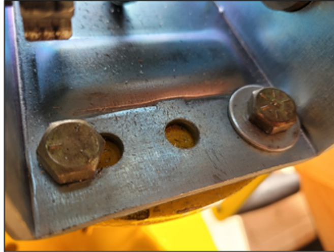
Figure 16: Winch-mounting Bolts Warped after Testing
