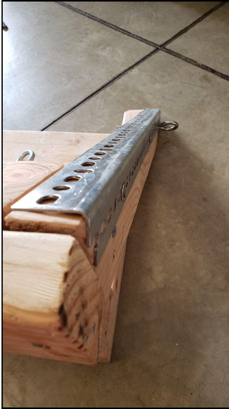
Figure 24: The rails that run along the bottom of the platform
