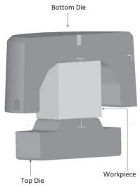
Figure 2 3D geometric model of pre-forge process
