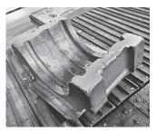
Figure 7 Railway wagon bogie adapter formed by forging
