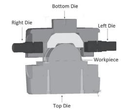
Figure 3 3D geometric model of final forging sequence
