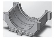
Figure 1 Schematic diagram of railway wagon bogie adapter product
