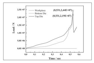
Figure 6 Load-stroke curve in forming
