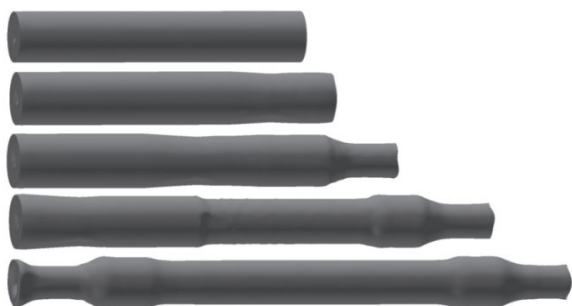
Figure 5 The rolling process of hollow axle
