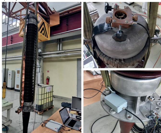
Figure 1: Electrical circuit configuration for frequency response check of the Končar TMS+ measuring system.
