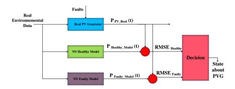
Figure 16. Descriptive schematic of the proposed FDD electrical-based in the PV generator.
