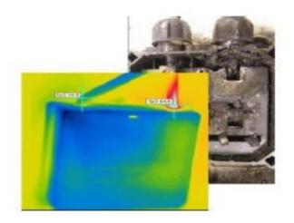
Figure 15. Example of fault in the JB: Corrosion.
