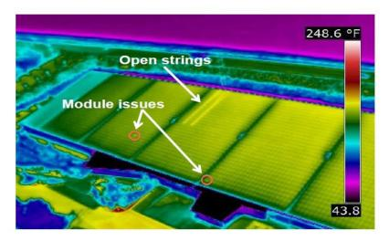
Figure 6. Example of Open-Circuit in a PV string (OC).
