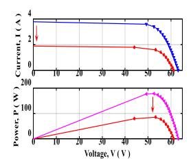
Figure 5. I-V and P-V characteristics with Open-Circuit fault effect.
