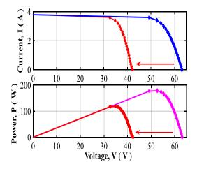
Figure 7. I-V and P-V characteristics with Short-Circuit fault effect.
