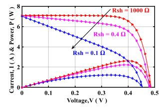
Figure 11. Effect of decreasing shunt resistance on the I-V & P-V characteristics.
