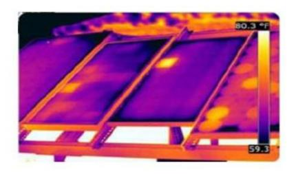
Figure 8. Example of Short-Circuited PV cell (SC).
