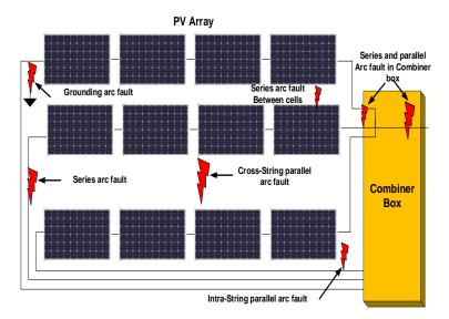
Figure 14. Descriptive schematic of Arc-Fault (AF).
