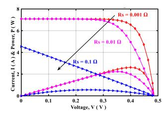
Figure 10. Effect of increasing in series resistance on the I-V and P-V characteristics.
