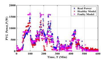
Figure 18. Real and modeled data for power, in a faulty PVG (shading a single PV module in the PVG) (26/10/2020).
