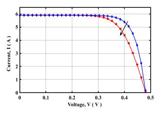
Figure 9. Effect of abnormal degradations in the I-V characteristic.
