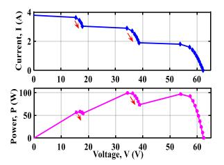
Figure 4. I-V and Power-Voltage (P-V) characteristics of PV generator with shading fault effect.
