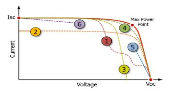
Figure 3. I-V curves under various types of faults.
