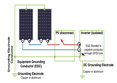
Figure 12. Descriptive schematic of a Ground-Fault (GF).
