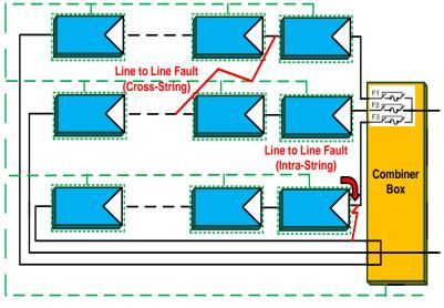
Figure 13. Descriptive schematic of Line-to-Line Fault.
