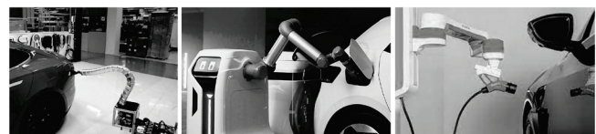
Figure 7 Selection of prototype systems for conductive side coupling. Left: Tesla charging snake [14]; middle: VW charging robot [13]; right: Kuka Carla charging connect [15]
