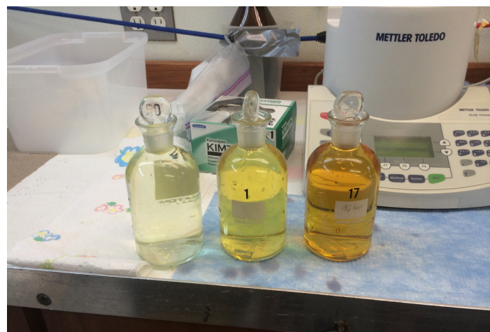
FIGURE 4. BOD (biological oxygen demand) bottles with fixed Winkler samples to be titrated to determine the dissolved oxygen (DO) concentration in mg/L. From left to right, the color of the sample indicates low oxygen to high oxygen concentrations. The potentiometric titrator is behind the BOD bottles.
