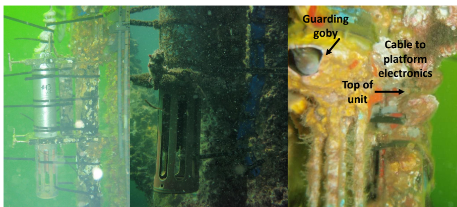
FIGURE 5. Levels of biofouling on YSI 6600 deployed oxygen meters. Left: newly deployed meter, no fouling, clean probe guard, and taped sonde unit. Center: a deployed sonde to be retrieved; the probe guard is clean, but the sonde body is becoming covered with barnacles. Right: heavily fouled sonde unit, oil platform leg on left, upper sonde on right.
