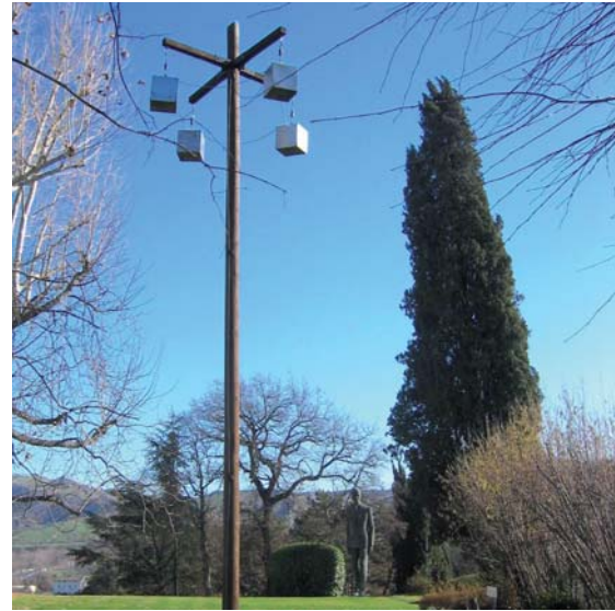
Figure 4a. A reconstruction of Marconi's 1895 antenna in the garden of Villa Griffone, Marconi's house (courtesy of Marconi Foundation).
