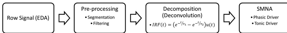
Fig. 2. Electrodermal acquisition and decomposition process. The EDA is filtered to reduce the noise and then decomposed in tonic and phasic components by means of a deconvolution with an IRF called the Bateman function.
