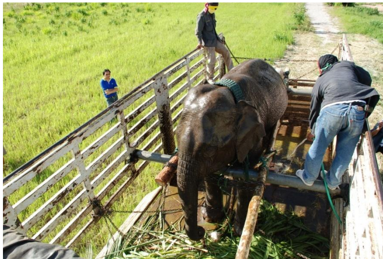
Figure 3: If the elephant is travelling by truck, a stall is built for it. (That stall can easily be dismantled and used again for the same type of truck: ten-wheel, six-wheel, etc.)
