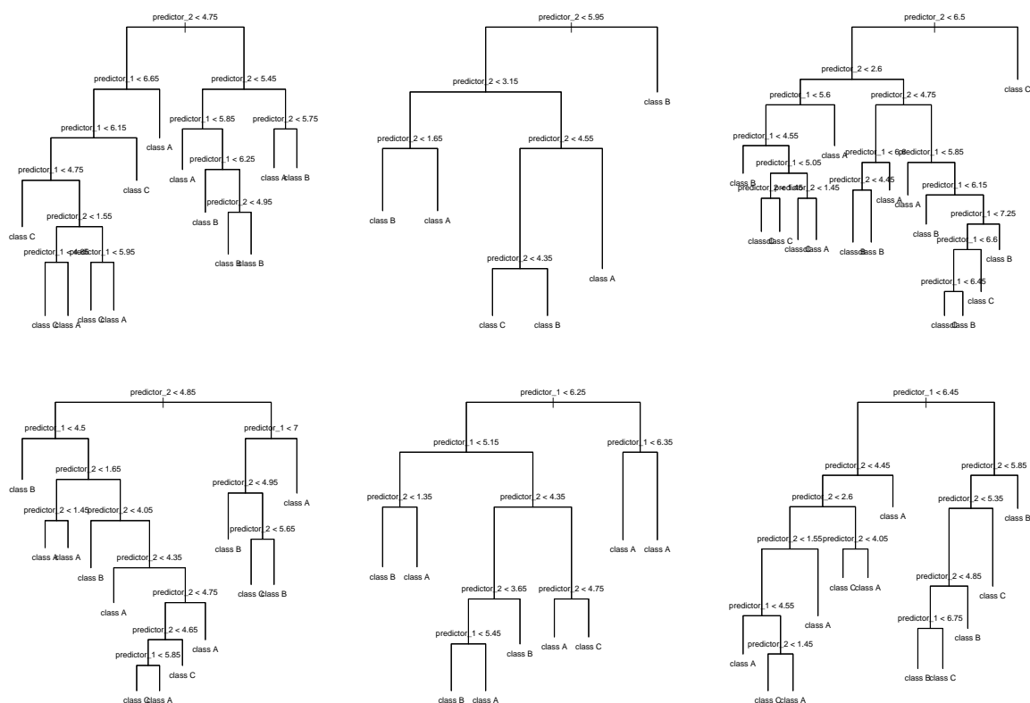
Figure 5.6: Example of a bagged ensemble of decision trees. Each tree in the ensemble is grown on a bootstrap sample of the original data. The large differences in the tree structures highlight well the high-variance nature of decision trees.
