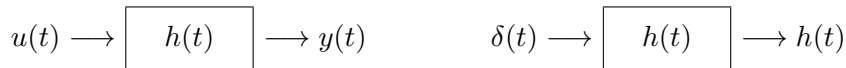
Figure 2: Schematic representation of a generic convolution operation, where u(t) represents the system input, y(t) represents the system output and h(t) is the IRF, depicted in the right-hand panel as the observed system output in response to a unit strength impulse, \delta(t) .
