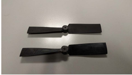
Fig. 6. 3D printed NACA proprotors.
