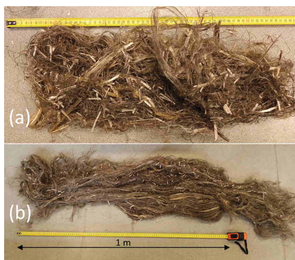
Fig. 2. Scutching tows: (a) mixture of shives, short and average length fibres; (b) Shives and long line fibres.
