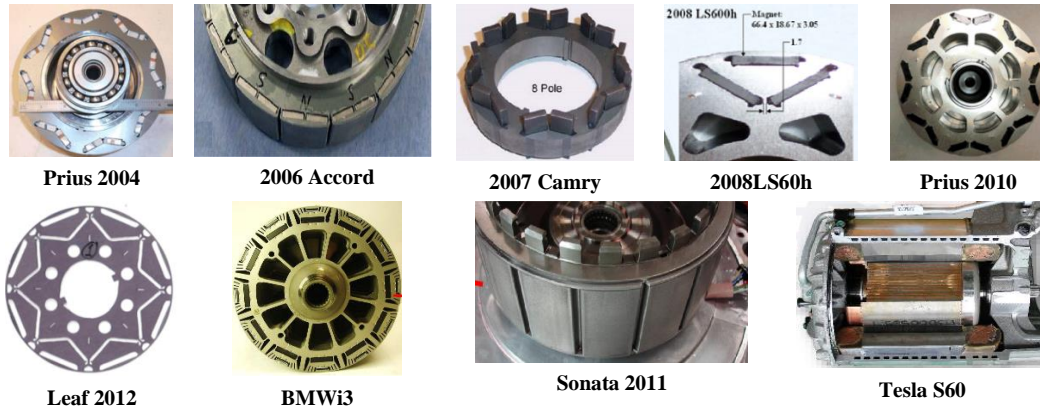
Figure I. 46. Rotor topologies of electric motors used in HEV [Hend_14] [Sar_17] [Sta_17]
