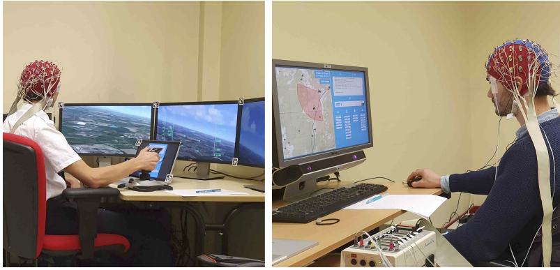
Fig. 1: Experimental setup: the Pilot (left) is flying the aircraft and exchanges instructions via a tablet with the JTAC (right) who is in charge of supervising the aircraft trajectory and gives instructions to the Pilot via the user interface.
