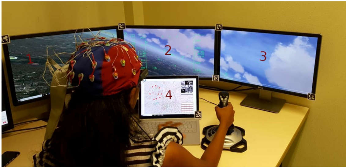
FIGURE 2 | Aerofly simulator and U-track application screens setup.
