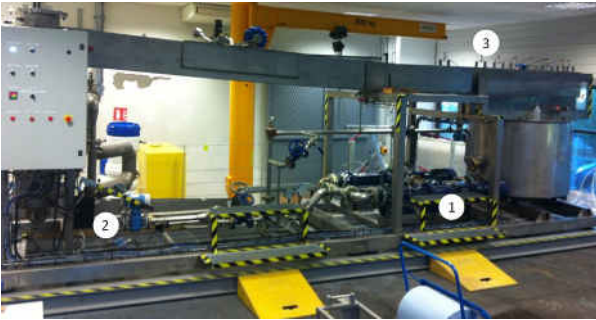
Fig. 6: Flow loop at Geoservices equipped with a Coriolis flow meter and eight ultra-sonic height sensors.
