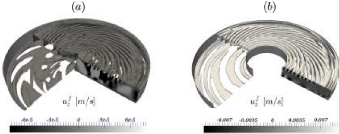
Figure 2.8 – Three-dimensional iso-contour of the axial velocity fluctuations u_z^f = u_z - \langle u_z \rangle of (a) Case 1 and (b) Case 2 complemented by a two-dimensional colour-mapping in a planar slice at \theta = 0 with associated colorbar.
