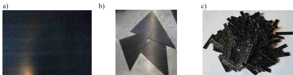
Figure 1. a) Initial laminate, b) Production scrap, c) aggregates.
