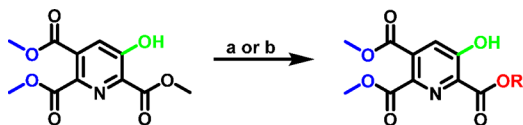
Scheme 22. Regioselective Transesterification: (a) 10 mol % \text{EtNiPr}_2 , ROH, 60 °C; (b) 5 mol % \text{Sc}(\text{OTf})_3 , ROH, cat. \text{H}_2\text{O} , 60 °C 208
