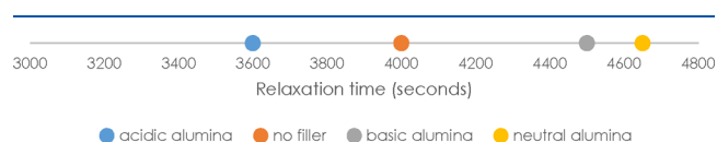
Figure 4. Effect of different functionalization of alumina fillers on vinylogous urethane vitrimer composites' relaxation time.
