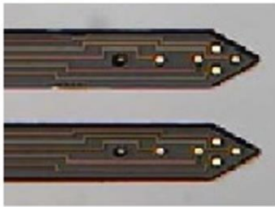
Fig. 5: Historical implantable MEAs types. (A) SEM picture of the recording tips of an Utah array, (B) SEM picture of the entire array, (C) Optical picture of two blades from a Michigan Array, (D) Optical picture of the entire array [27], [26] (modified), [28].
