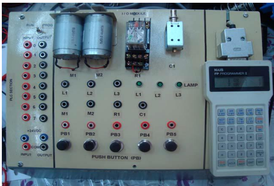
Figure 2.1: Overall view of PLC Kit
