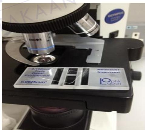
Figure 3.3: Compound light microscope and haemocytometer grid chamber
