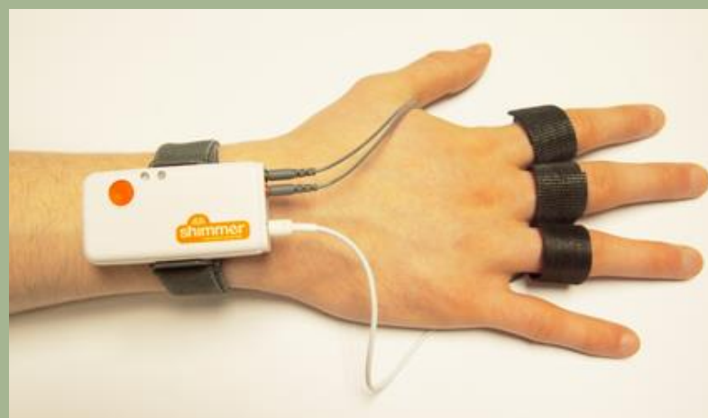
Figure 2. GSR unit with electrodes for skin conductance and skin temperature measurements and photoplethysmography sensor for heart rate recordings.
