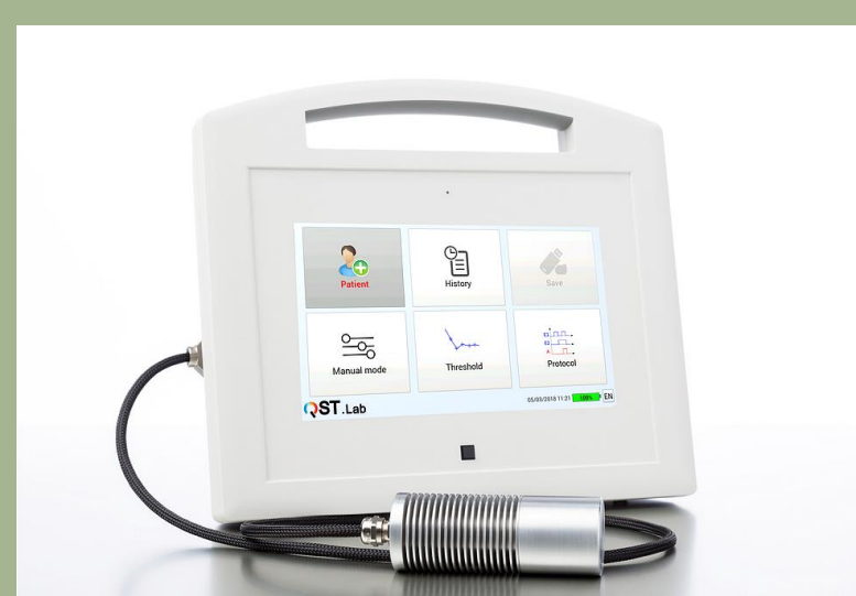
Figure 3. Thermode control panel and trigger to apply quantified thermal pain stimulus.
