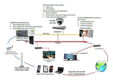
Fig 5: Intruder Alarm and Detection System
