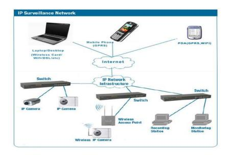
Fig 2: IP Surveillance Network
