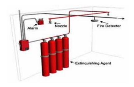
Fig 3: Fire Detection and Alarming system
