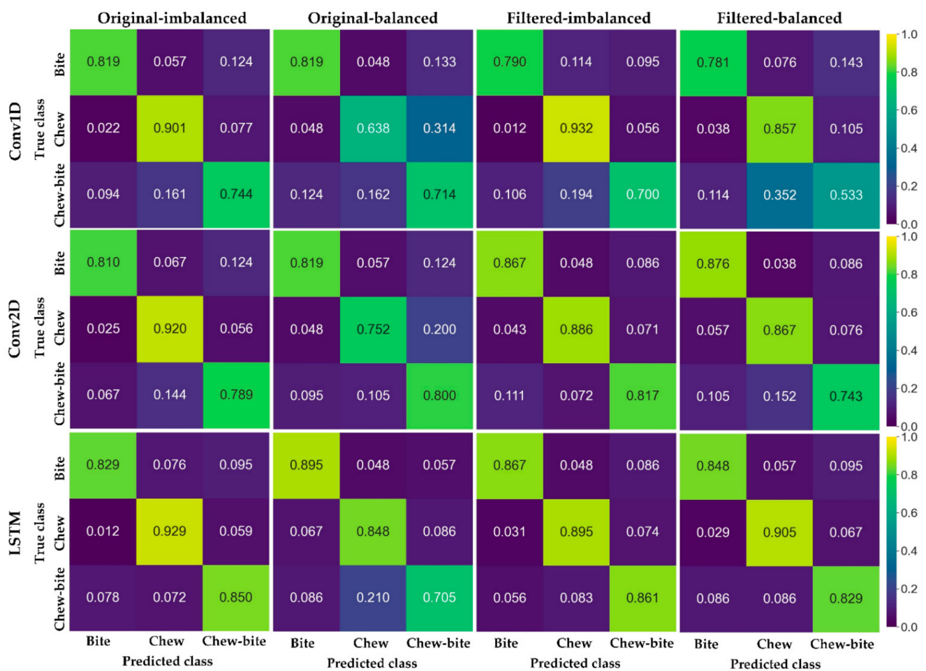
Figure 8. Confusion matrixes of the three deep learning models for classifying the ingestive behaviors in various datasets. Conv1D represents one-dimensional convolutional neural network; Conv2D represents two-dimensional convolutional neural network; and LSTM represents long short-term memory network. “Original” indicates the original dataset without any filtering; “Filtered” indicates the dataset was filtered with the bandstop filter to remove background beeping sounds; “imbalanced” indicates the dataset with unequal audio file sizes for the three ingestive behaviors; and “balanced” indicates the dataset with equal audio file sizes for the three ingestive behaviors.
