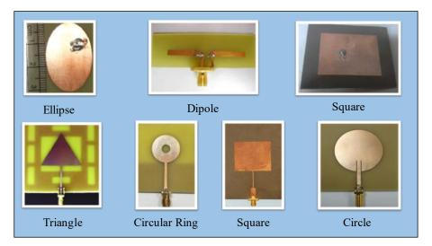
Figure 3: Different Shapes of Microstrip Patch Elements.
