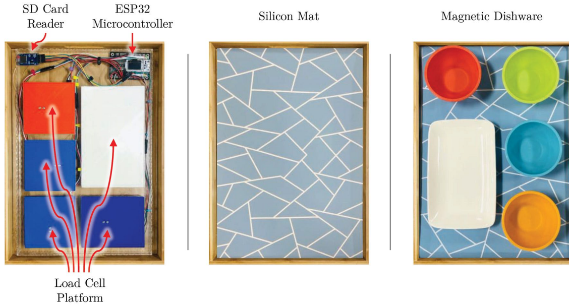
Fig. 1. The three layers of the tray (electronics, protective silicone, dishware).
