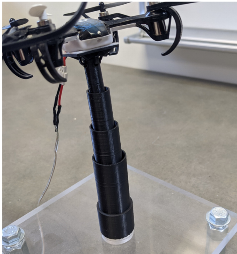
Figure C.1: A telescopic mount for the TAUS-Alpha Holy Stone micro-UAS. This was developed and integrated so we can test various power demands based on actual throttle, roll, pitch, and yaw commands.
