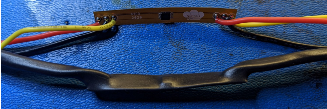
Figure 3.10: Version 2 of the flexible PCB with the sensor IC soldered in place.
