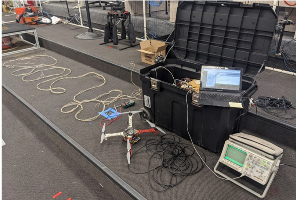
Figure 3.7: The TAUS-Beta initial power and sensor array integrated tether developed for laboratory testing.
