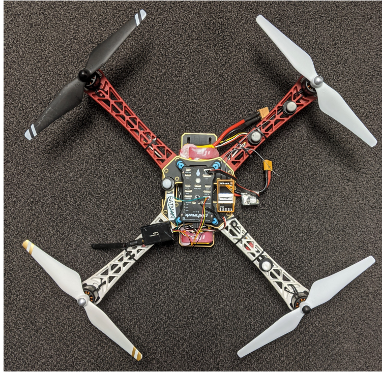
Figure 3.1: DJI flamewheel f450 with mounted Pixhawk
