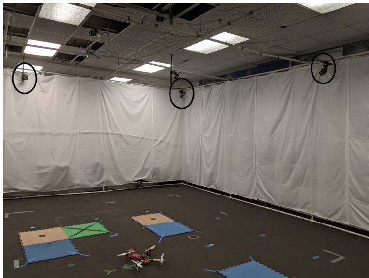
Figure 3.2: View of NIMBUS Lab testing space with some Vicon cameras circled
