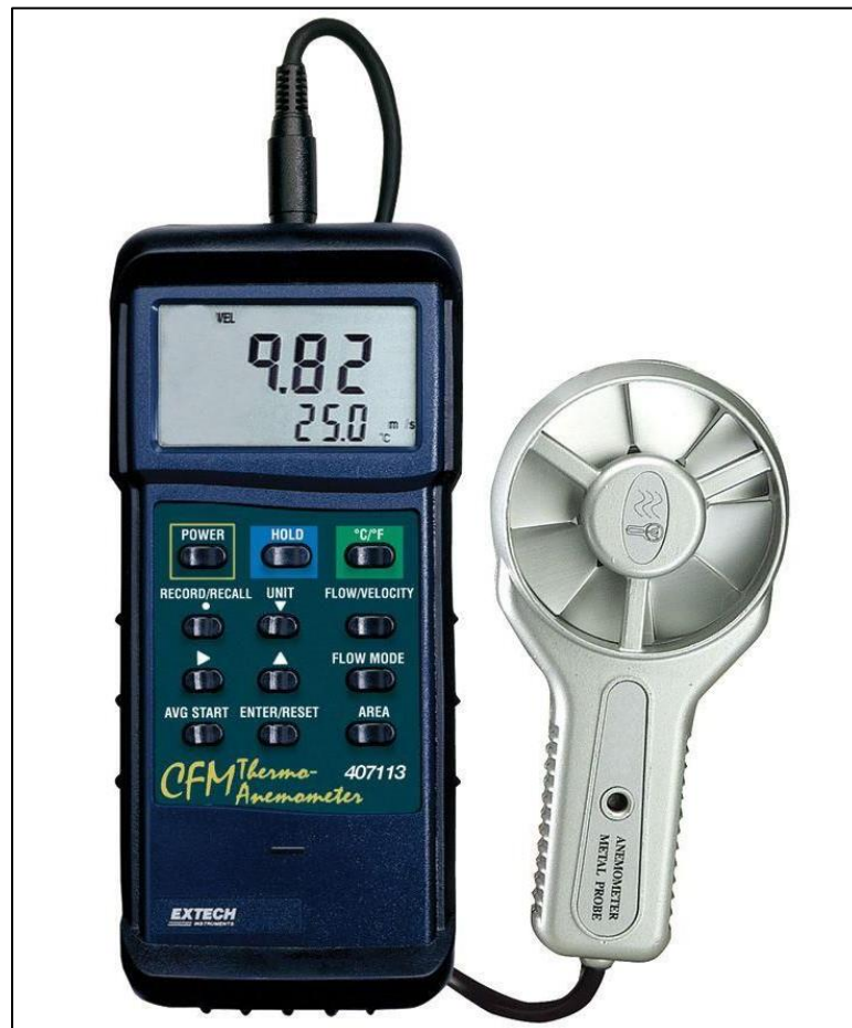
Figure 12. Electric high temperature metal probe anemometer.
