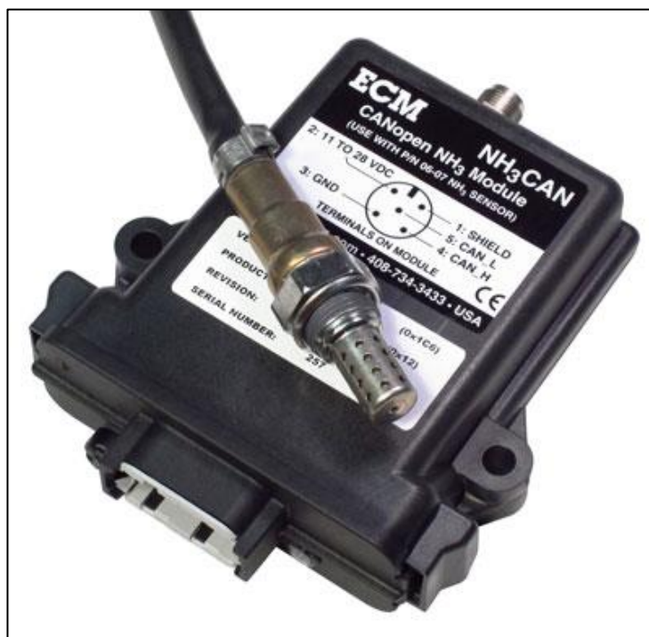
Figure 11. The NH 3 CAN Module of the ECM miniPEMS.
